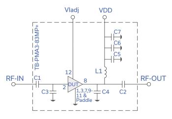
Fig 1. Application and Characterization Circuit
